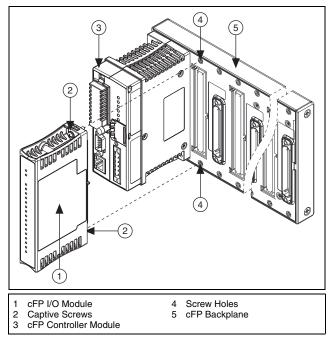
Figure 2. Installing the cFP-PWM-520
